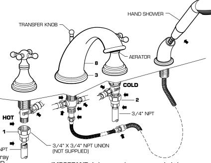
IMPORTANT: It is strongly recommended that access be provided for all enclosed mechanical parts to this system.
